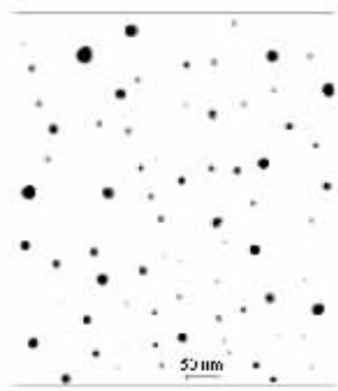
Fig. 3 TEM image pattern of Pr 2 S 3 nanoparticle.
